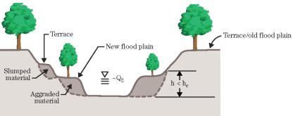
Figure 17. Conceptual model of incision channel evolution by Schumm et al. (1984). Reprinted from USDA NRCS (2008).
